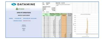
Once cut & fill volumes have been created, you can publish the results to a summary Excel spreadsheet (again, using a custom template) and analyse month-end results. In addition to the above, Studio Survey users have access to a wide range of Studio Core functionality to make digitizing, designing, presenting and analysing survey data easy.
